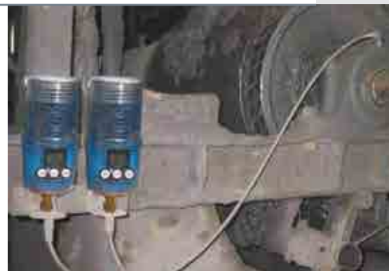
Remote-mounted Lubri-Cup™ EM dispensers for hard-to-reach areas on the head pulley.
